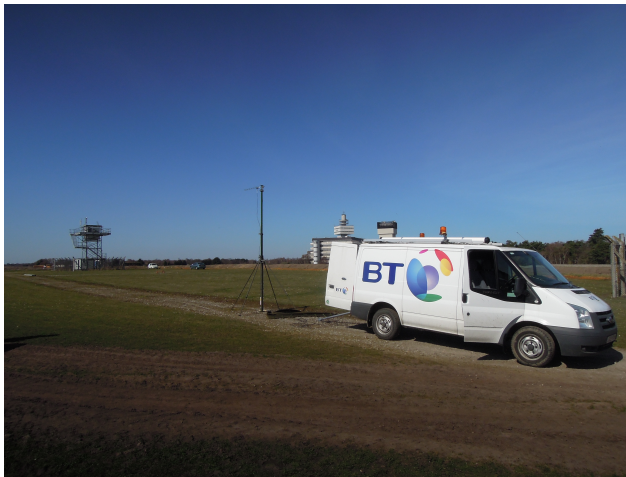
Figure 6.5: Measurement van and Yagi antenna.
